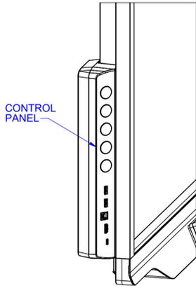
DETAIL A - (ISOMETRIC) LEFT CONTROL PANEL
