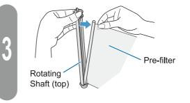
Pull out the Pre-filter from the Rotating Shaft (top)
