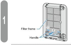
Move the handles (left and right) in the direction shown in the picture(1) and take out the filter frame(2).
