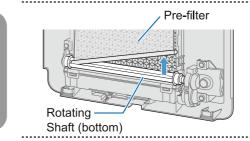
Pull out the Pre-filter from the Rotating Shaft (bottom)
