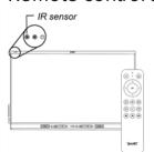
You can use the remote control to turn the display on and off, adjust display settings, and so on.
