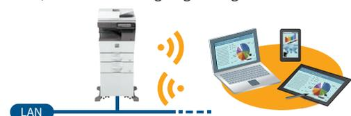
Note: External networks cannot be accessed via the MFP. Up to five mobile devices can be wirelessly connected to the MFP at the same time.
