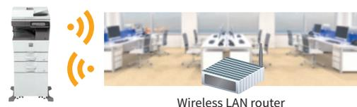
• **Access Point mode** wirelessly connects a LAN-wired MFP to mobile PCs/devices without going through a wireless LAN router.
