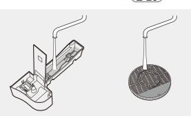
Whether the Filter Maintenance Indicator is lighted on or not, it's better to clean and wash the Humidifying Filter and the Tray thoroughly so that mineral substances have less chance to attach on the surface of the Humidifying Filter and thus inhibits the generation of odor.
