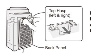
Remove the back panel and take out the filters.
