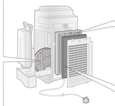
Please clean and maintain the HEPA Filter and 2-in-1 Deodorizing & Deformaldhyde Filter when there is odor blowing out from the air outlet and it is hard to get rid of it.
