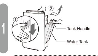
To remove the Water Tank, please push down the Handle and pull outwards.
