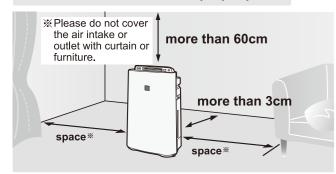
\*\* The dust collection ability will not be affected even if the unit is located within 3cm from the wall; however, the wall and the ground may be dirted, therefore, please keep the unit as far as possible.
